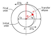
During the transfer the Earth moves by  $180^{\circ} + \theta = 257^{\circ}$ , so the spacecraft should launch from Mars when Earth is at position A" (exhibiting symmetry with when it arrived).
