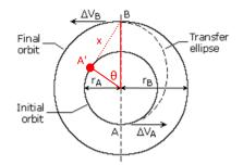
Initially Earth is at A. When the spacecraft reaches B (after 8.56 months), the Earth has moved round the Sun in its orbit and is now at A'.
