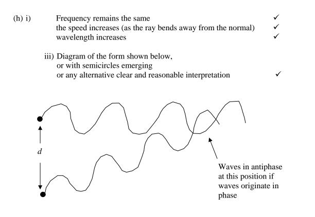
iii) minimum *d* is  $d_{min} \approx \lambda/2$   $\checkmark$  orientation: the two waves are collinear with the centres of the speakers  $\checkmark$  (6 marks)
